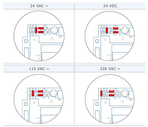
The output voltages 115Vac or 230Vac is not available in 24Vdc power input models.
