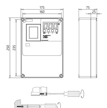
12-16 Outputs Enclosure Dimensions in mm
