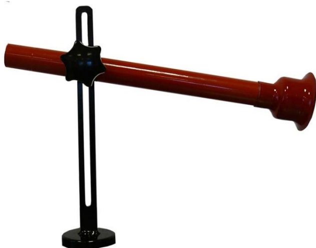
Photo No.1 – Nozzles for fume extraction for point welding and longitudinal welding
