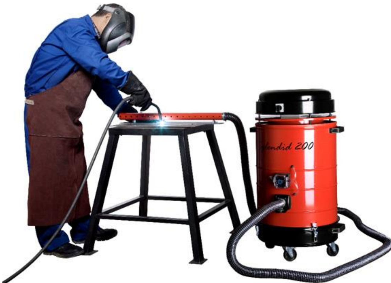
Photo No.2 – Example of application of the device for longitudinal welding
