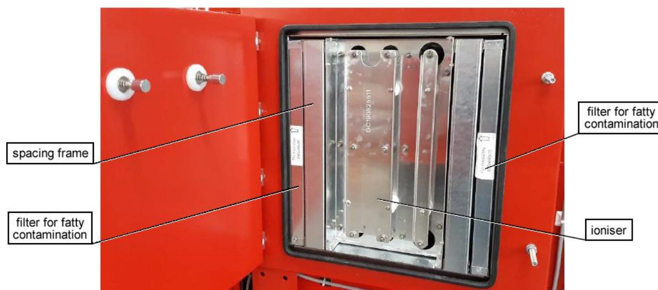
Photo No.2 – Filtration chamber – inside
