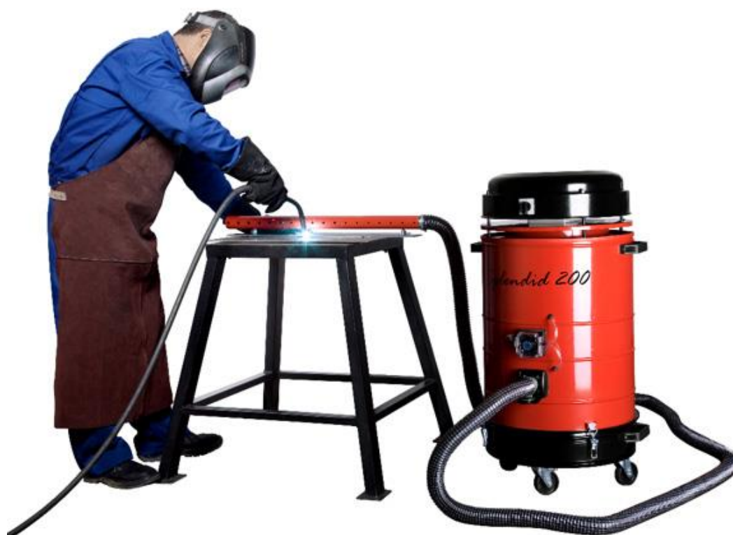
Photo No.3 – Example of application of the device for longitudinal welding
