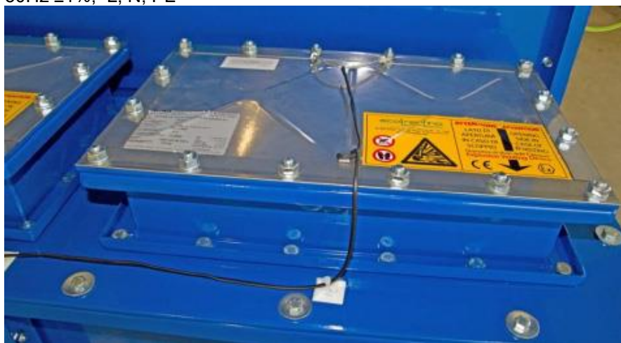
Fig. No.13 – Decompression panels
