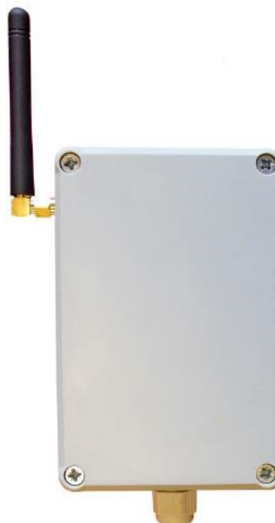
Fig. No.9 OR-1 radio receiver
