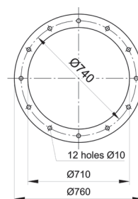
Sound absorbing roof base TPDC-710-N
