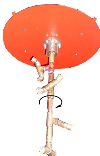
Phot. No.3 System of automatic filter cleaning
