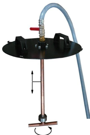
Phot. No.2 System of manual filter cleaning
