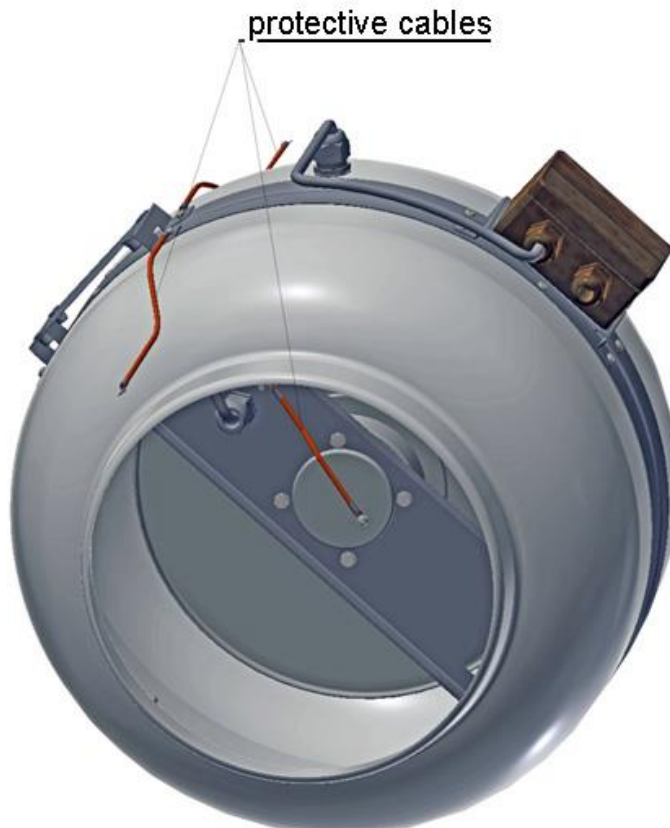
Fig. No.3 – Protective cables placement
