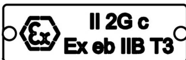
Fig. No.4 – Nominal data plate and explosion-proof plaque
