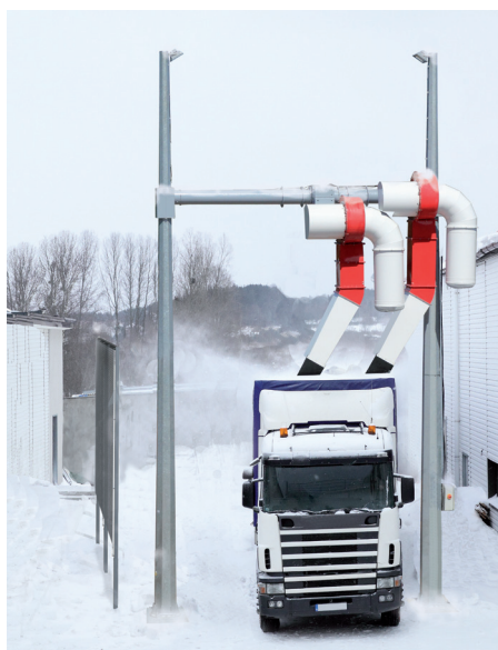
SNOW OUT TRUCK during the operation
