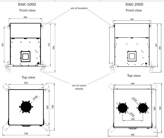
NOTE: Broken line illustrates the elements of additional equipment.
