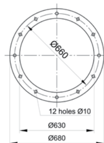
Sound absorbing roof base TPDC-630-N
