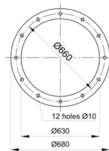
Sound absorbing roof base TPDC-630-N
