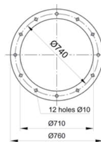
Sound absorbing roof base TPDC-710-N
